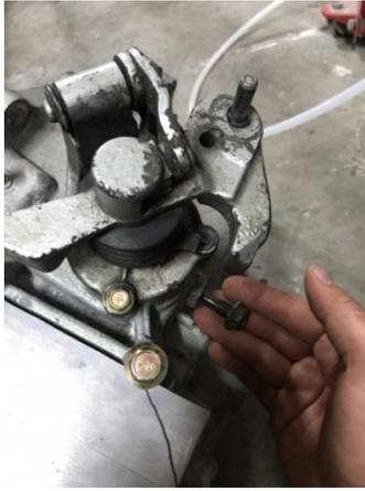
Now, there are 4 bolts that attach the shift selector assembly to the transmission. They can all be accessed from the top with a 10mm socket and extension. You may need to move the shift arm to various positions in order to gain access to every bolt.
