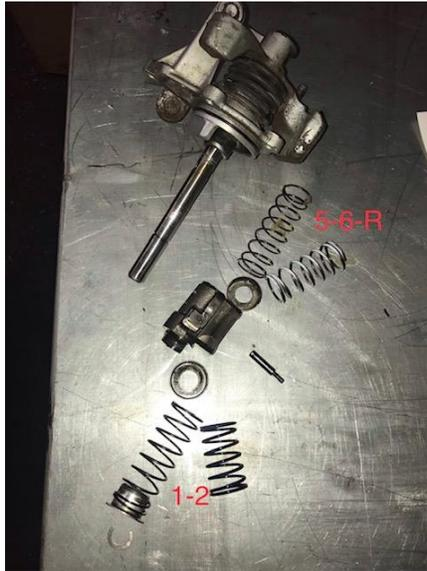
Replace the upper 5-6-R spring (longer of the two) with the white 5-6-R spring (longer of the two) provided
