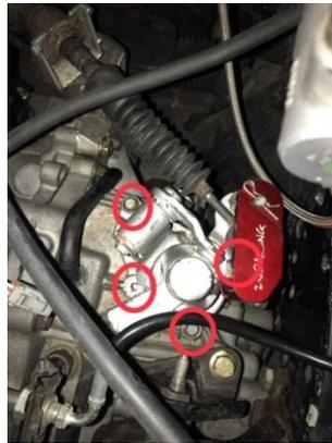
After the four 10mm bolts and the 14mm plug are removed, you'll be able to pop the shift selector assembly out the top of the transmission.
