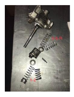
Replace the upper 5-6-R spring (longer of the two) with the black 5-6-R spring (longer of the two) provided
