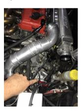
Next, you'll use a 14mm wrench to remove the shift change pin on the driver side of the transmission just below the shift selector assembly. This simply looks to be a 'plug' with a 14mm hex head.
